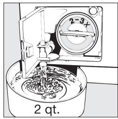
■ Turn the lint trap lid counterclockwise 2 - 3 times. Do **not** remove it. Approx. 2 quarts (2 l) of water will drain out of the hose.
